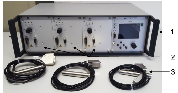
Figure 7 Piezo system 1: Digital piezo amplifier 2: 3x LVPZT modules EVD300 3: 3x piezo actuators PA 70/14 SG
